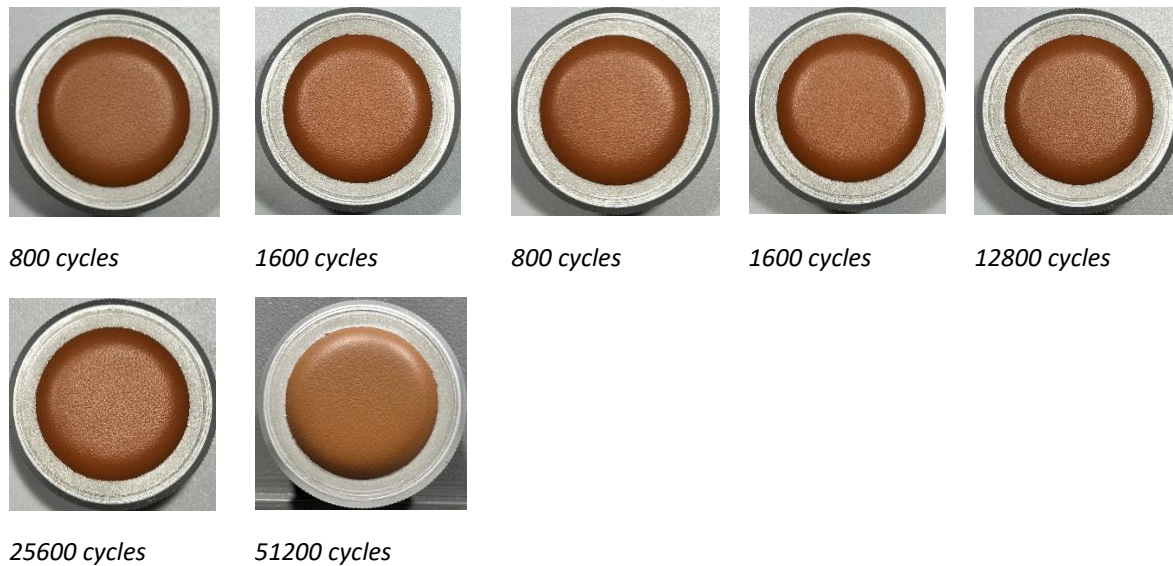
Fig. 16 – Leather for iPhone casing Martindale abrasion test
